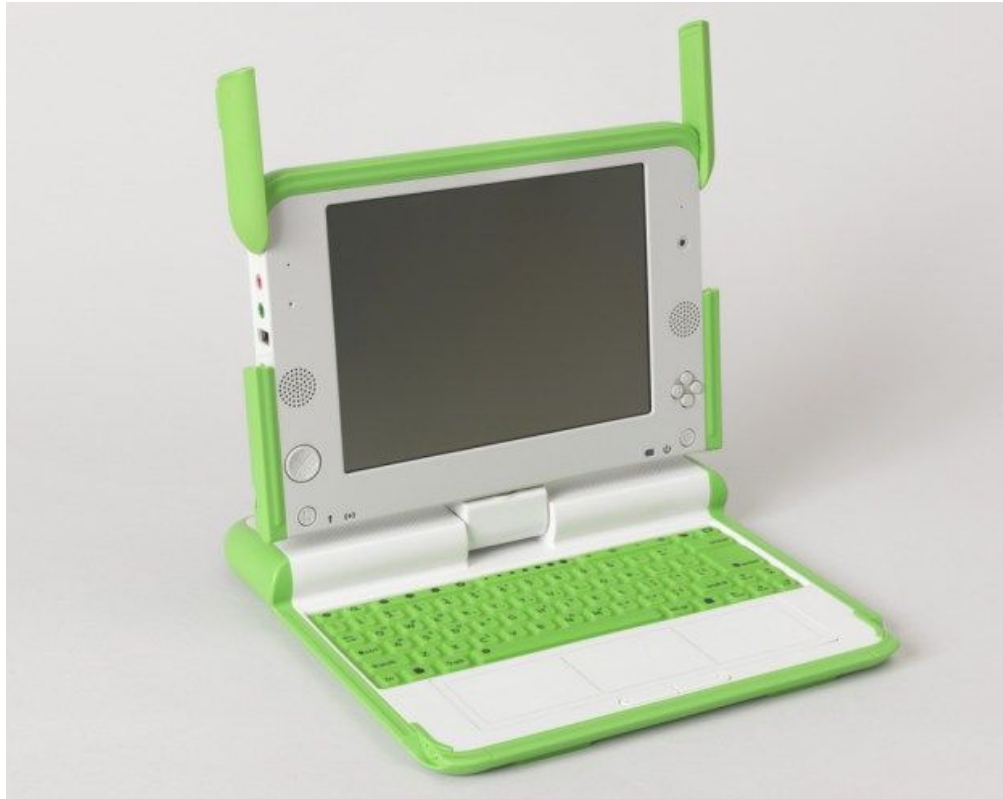
One Laptop Per Child XO Computer, 2007; Designed by Yves Béhar, Bret Recor and fuseproject; injection molded abs plastic and polycarbonate, printed rubber, liquid crystal display, electronic components; steel, copper wire (power plug); H x W x D (closed): 3.5 x 22.9 x 24.1 cm (1 3/8 in. x 9 in. x 9 1/2 in.); Gift of George R. Kravis II; 2015-5-8-a,b; Object Record
